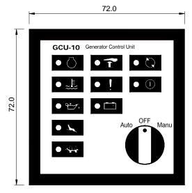
Cut-Ou  $66.0\pm0.5 \text{ mm} \times 66.0\pm0.5 \text{ mm}$
