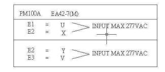
Original PM100 is used in 1 or 3 phase alternators. If used with 3 phase sensing voltage feed lines into E1, E2, E3 (one E2 lead is null)
