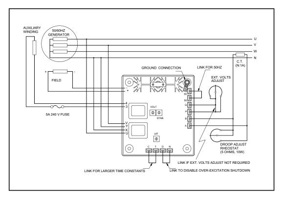
Figure 2-2 Interconnection Diagram, 480 Vac High Y Generator.
