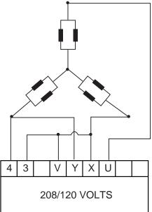
INPUT TERMINALS 3 & 4 CAN BE POWERED USING THE GENERATOR ITSELF, AN AUXILIARY WINDING OR A PMG. THE INPUT OF 3 & 4 MUST BE
