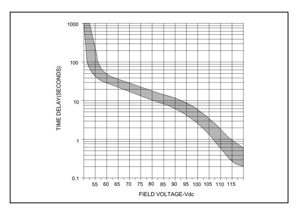
Figure 1-2 Typical Inverse Time Delay Characteristic Curve.
