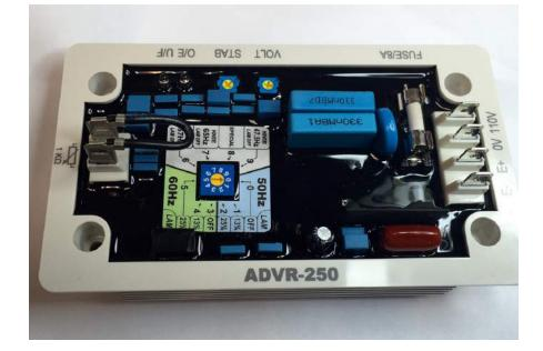
Analog / Digital · Single-phase detection · Excitation Current 3.5 Amps. For use in brushless, self-excited (shunt) generators Compatible with Leroy Somer\* R250/R230, AVR
