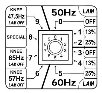
Warning!! The switch setting must correspond to the rated frequency. An error in settings could cause damage to the generator.
