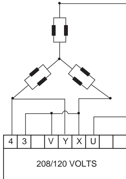
INPUT TERMINALS 3 & 4 CAN BE POWERED USING THE GENERATOR ITSELF, AN AUXILIARY WINDING OR A PMG.
